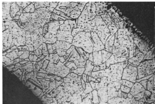
Fig. 4 Optical micrograph showing the tube wall (sample 16 tested for 20,000 hr, 50 \times ).
